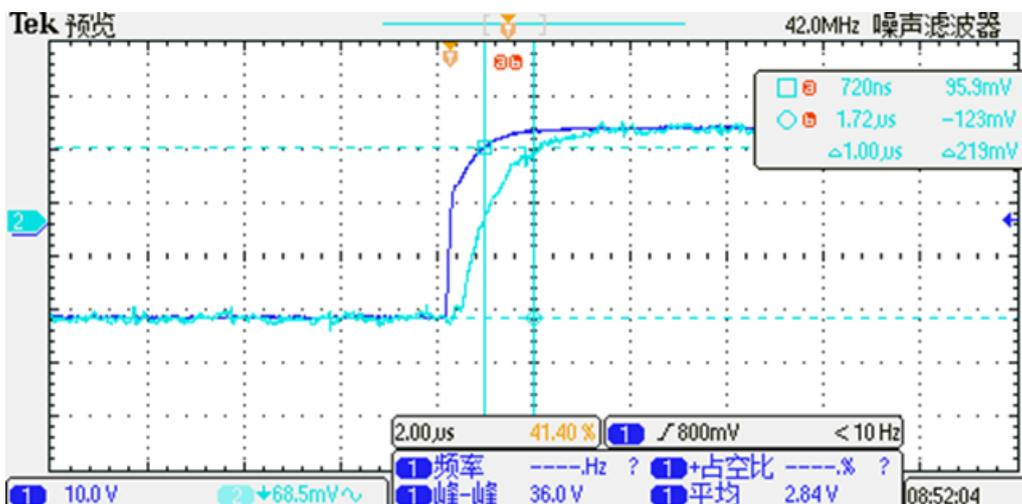
The typical low frequency response of STK-616YML current sensor. The response time from 90% of the primary current to 90% of the secondary output is 1μs.
