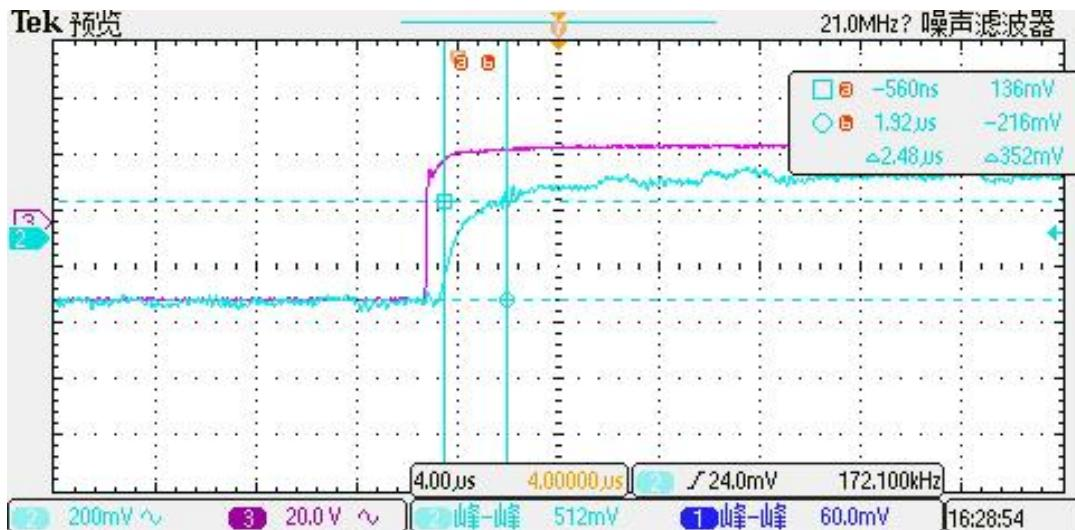
The typical frequency response of STK-616Y current sensor. The response time from 90% of the primary current (pink) to 90% of the secondary output (blue) is 2.48  $\mu$ s.
