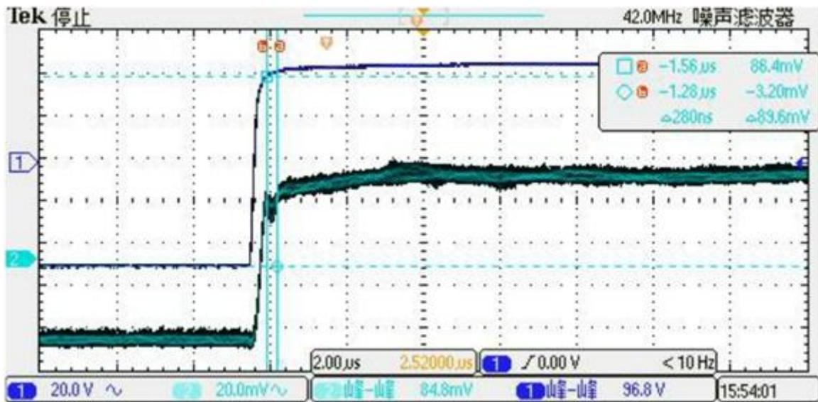
The step response time of STB-xxCAS/F current sensors. The blue is primary current, while the green is output signal of current sensor. The step response time is less than 0.3 μs.
