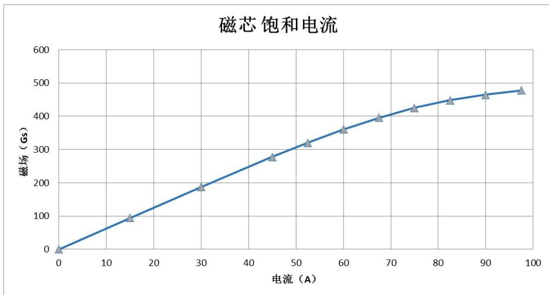
Test conditions: Gauss meter is used to test the open-gap magnetic field of the core varying with current.
