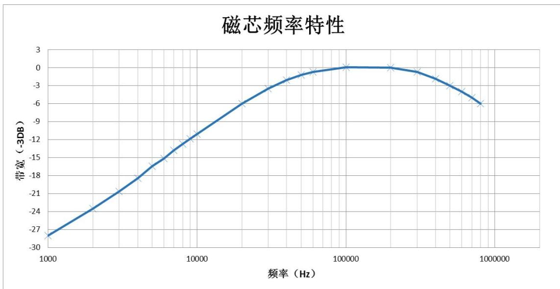
Test conditions: the current at the primary side is 10 mA, the sampling resistance is 100 ohm, and the amplification is 150 times. The output at both ends of the test resistance varies with the current frequency at the primary side. The cut-off frequency is calculated according to the volt frequency characteristics.
