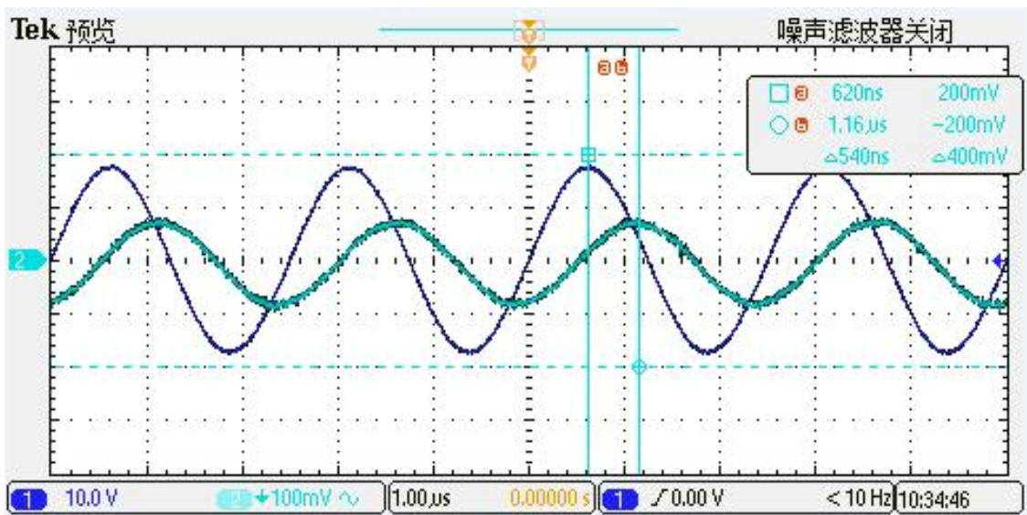
Remark: Primary current was detected at a frequency of 400 kHz. Typical results of stK-CTS /C current sensor output main current delay characteristics .
