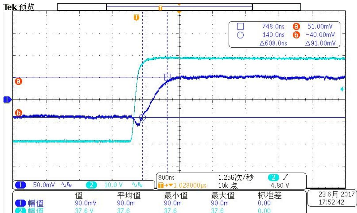
Remark: Step response time of STK-CTS/C current sensor. The delay from 90% of the original current signal to 90% of the sensor output is less than 1 us. .
