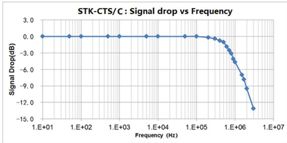
Remark: STK-CTS /C series current sensor bandwidth. The bandwidth of the sensor is in the range of DC ~ 400 KHZ (- 3db).
