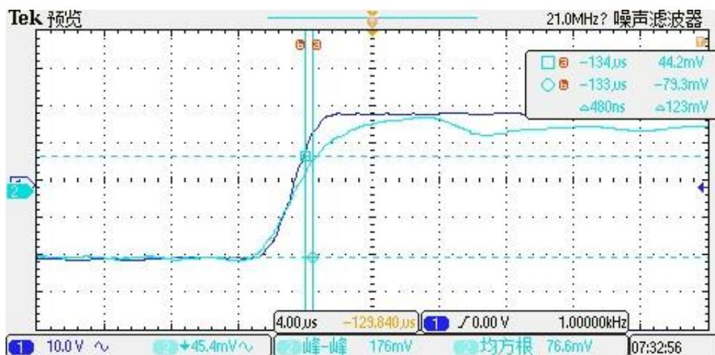
The step response time of STB-xxCAS/FA current sensors. The blue is primary current, while the green is output signal of current sensor. The step response time is less than 0.3 µs.
